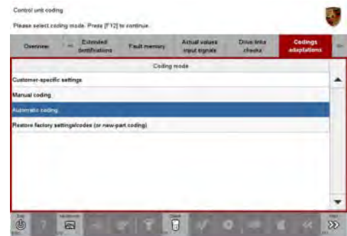
Instrument cluster - Automatic coding
