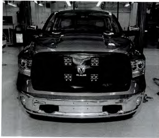
Fig. 3 Winter Front Cover Installed
