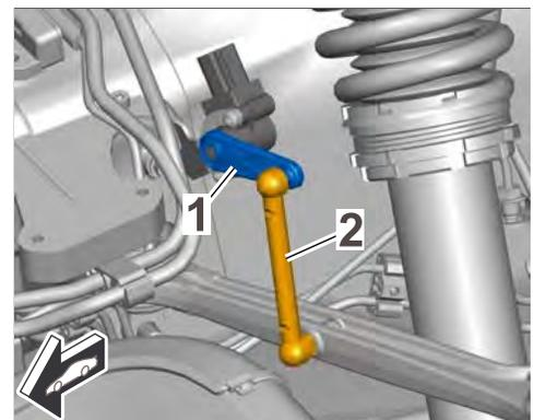
*Checking the level sensor for damage*
