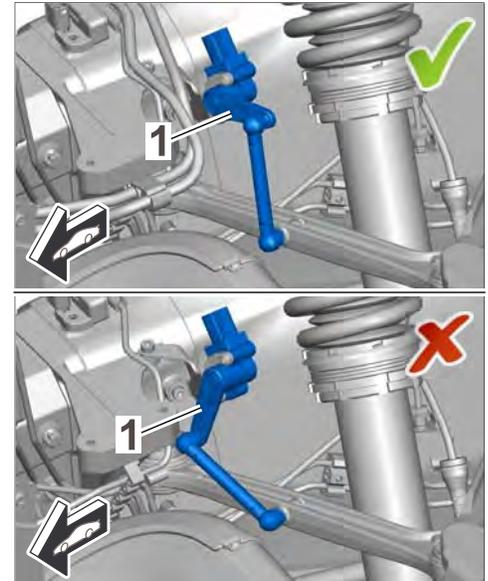
*Installation position of the level sensor*
