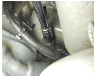
Insert the new screw (p/n 470198317) and fasten without tightening it.
