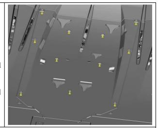
Detect the screw to be replaced: lower screw of starter motor.
