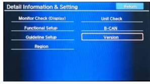
19. Verify that the software was updated to the new version as shown below. If the software is not updated, turn the vehicle to the OFF mode, and go back to step 2 and repeat the update procedure. *Accord*
