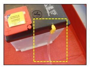
2. Remove the elbow from the vent hose.
