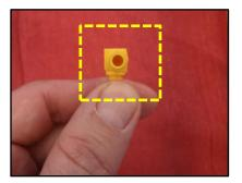
4. Use the side cutters to trim the end of the vent hose by 6mm (1/4") mm.
