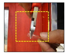
5. Install the vent elbow onto the vent hose. **Note: Make sure the modified end of the elbow is installed into vent hose.**
