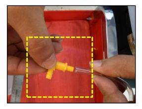
6. Reinstall the vent hose assembly into the vent hole nearest the positive terminal of the replacement battery.
