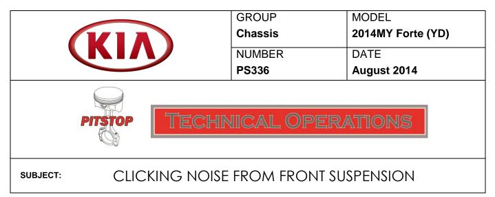
Some 2014MY Forte vehicles, manufactured prior to September 2013, may exhibit a clicking type noise from the front suspension when carrying a full load of passengers and turning the wheel in either direction at low speeds; such as in a parking lot situation or when pulling into steeply inclined driveway. To correct this condition, place the vehicle on the lift, raise the dust cover and apply a generous amount of silicone based lubricant onto the left and right strut caps, as shown below.
