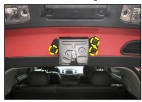
2. Shift the latch as far to the left as possible and re-torque the bolts to proper specifications. **Tightening torque:** 5.1~8.0 lb-ft (6.9~10.8 Nm).
