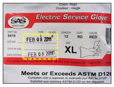
If the glove package has <u>NOT</u> been opened (i.e. still sealed) – the gloves <u>MUST</u> be recertified when beyond one (1) year from the date code stamped on the label.
