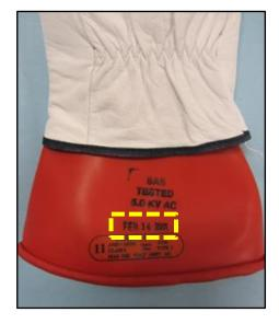
If the glove package has been opened – the gloves <u>MUST</u> be recertified once six months have passed from the date stamped on the glove and every six (6) months, thereafter.
