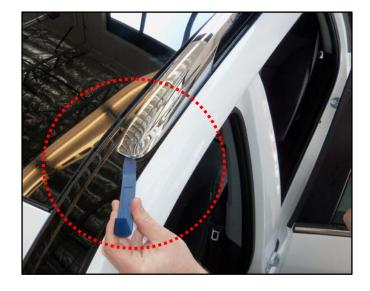
3. Carefully remove the rear sunroof side molding panel.
