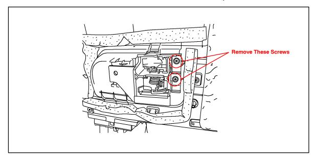
3. Install the NEW inside door handle assembly in reverse order and reassemble the door panel.
