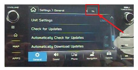
1.6.1) Wait until the download progress reaches 100%. During the software download, the H/U is fully functional. **NOTE:** It is normal for the progress to hang at some points for 1-2 minutes. This does not indicate a concern. **BE PATIENT**.
