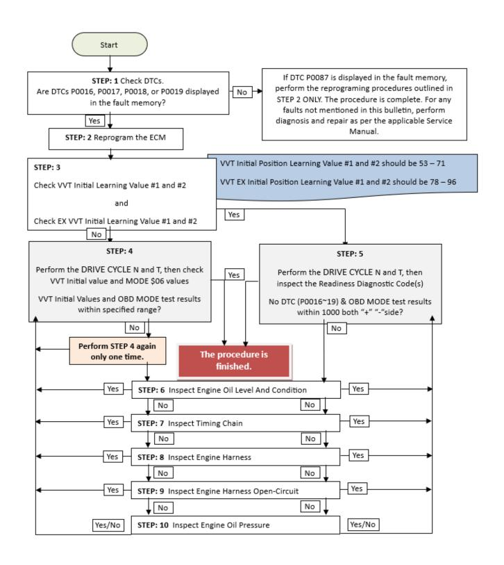
(\*1) Use the following instructions to perform and read the OBD MODE test results. This procedure will be required when performing the diagnostic steps outlined below.
