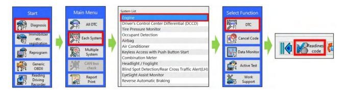
**P.** Read the readiness codes for P0016, P0017, P0018, P0019, P000A, P000B, P000C, and P000D. Confirm the self-diagnosis is complete and that the codes are not pending.
