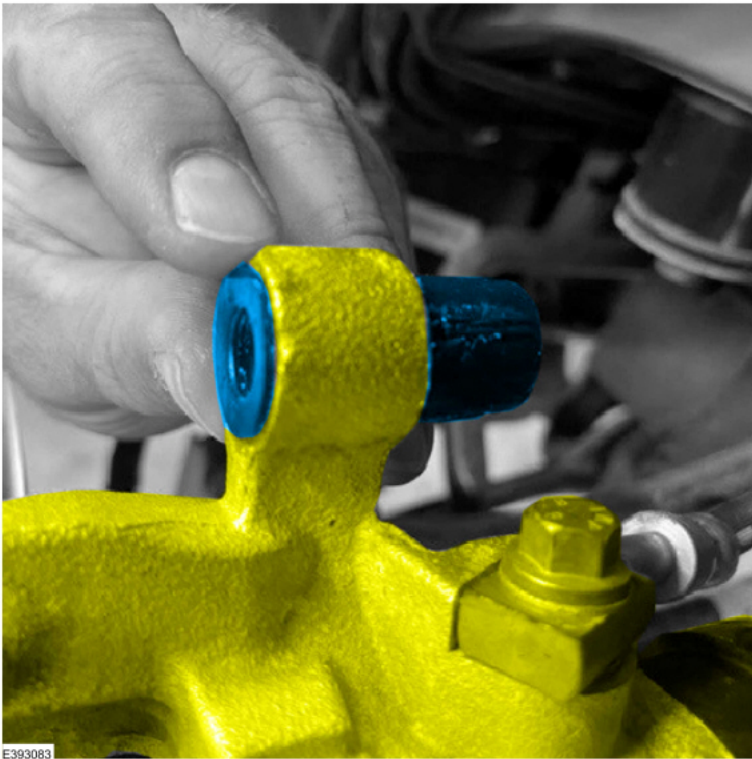
9. Position the rear caliper in place and install a new guide pin. (Figure 15)
