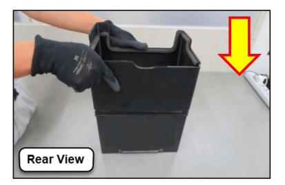
**STEP 5:** Assemble the new battery holder (**p.n. 82184SG000**), **NEW** rear holding rod (**p.n. 82161SJ000**), and the **ORIGINAL** front holding rod as shown below. The original rod nut can be transferred to the new rear holding rod.
