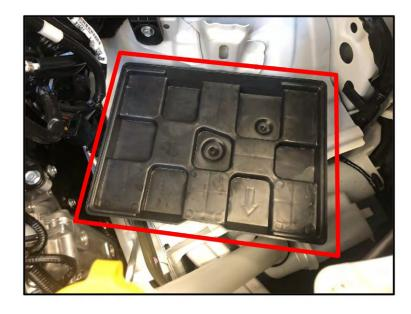
STEP 3: Replace the original battery tray with the new part (p.n. 82190AN000).
