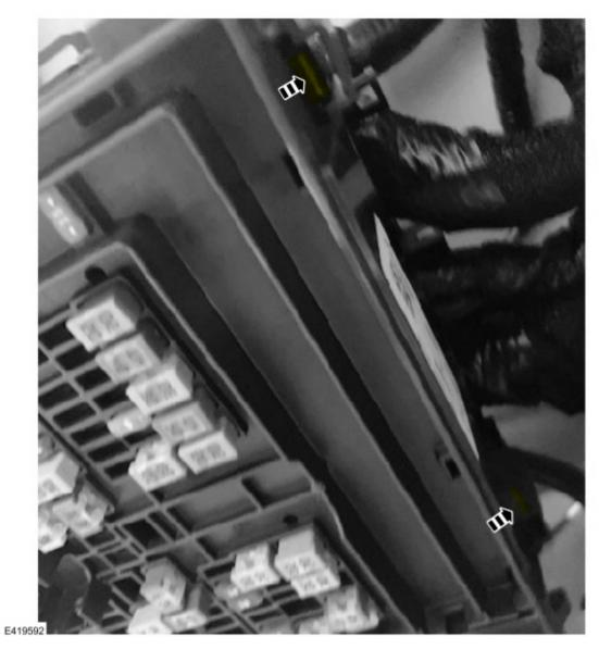
$\textbf{5.} \ \, \text{Lift the BJB from the bracket and remove the 3 wiring harness connectors. (Figure 5) }$  Figure 5
