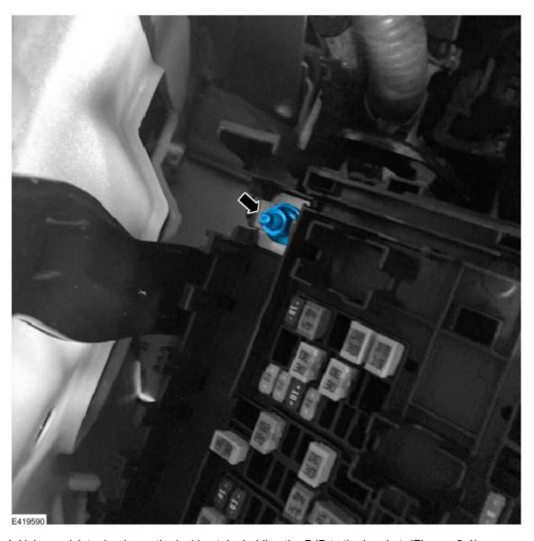
**4.** Using a pick tool, release the locking tabs holding the BJB to the bracket. (Figures 3-4) Figure 3
