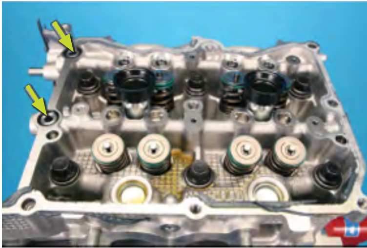
Cam carrier o-rings requiring replacement
