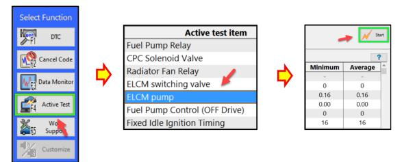
Once the ELCM Pump Active Test has been performed for a period of 35 minutes or more, repeat the Evaporative System Leak Test outlined in STEP 4. Check the DTCs and the vacuum value results.
