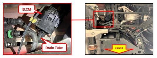
Have signs of water or oil been detected within the ELCM drain tube?
