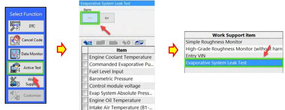
Once the evaporative system leak test is complete, check the DTCs and examine the vacuum value results. Record the value shown in the row labeled MID: \$3C, TID: \$C4, and Scaling ID: \$FE. This value should be lower than -0.26 PSI.
