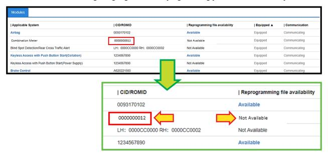
**STEP 22)** Once the updated CID/ROMID is visible on the Vehicle page and no other updates are to be performed, the user must first close BOTH the SSM5 web browser page first and then the Cloud Connector application to ensure the next user is not logged into the current user's account.
