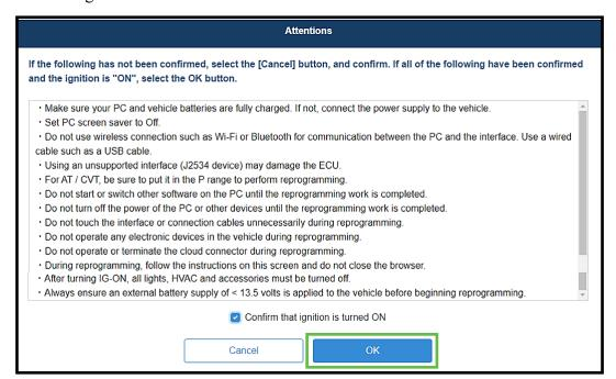
STEP 13) Reprogramming will now start. NEVER disrupt or close the web page or the Cloud Connector, disconnect any cables, power off the interface, or disturb the process in anyway during the reprogramming process. During this step, the .pfc file will be retrieved from the cloud server.
