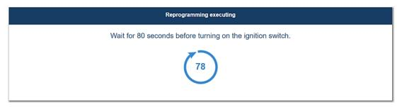
**STEP 18)** When the timer has reached zero, a new pop-up window will appear. Confirm the ignition in the "ON" position by checking the box and clicking "OK".
