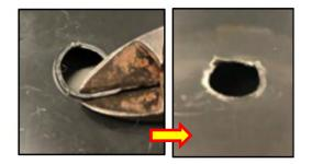
**CAUTION:** Be sure the protrusions are trimmed flush. The remaining protrusion height MUST be less than 2mm to provide proper fitment.
