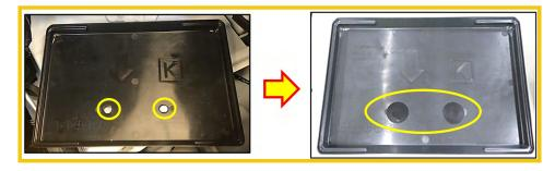
**D.** Securely fit the replacement battery tray to the vehicle.
