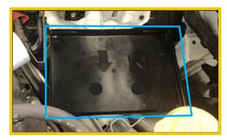
STEP 4: Install the NEW battery cover (p.n. 82123AN000) to the alternative replacement battery. Confirm the bottom of the cover is aligned flush with the bottom of the battery.
