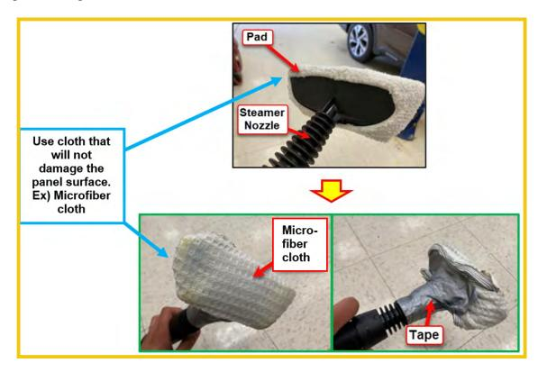
**STEP 3: CAREFULLY** apply steam to the affected area evenly for three minutes. A timer can be used to ensure the proper time frame. Using an infrared laser thermometer, monitor the temperature of the painted surface. The recommended temperature is 176°F (80°C) to 194°F. **NEVER** exceed 212°F. Allow the affected area to cool, dry and inspect the surface. Repeat this process up to **THREE** times if discoloration and swelling is still detected.
