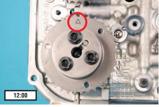
• Align the indicator link with the timing mark on the crankshaft sprocket as shown below.
