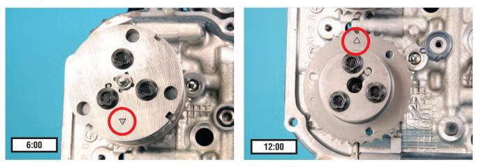
• Align the indicator link with the timing mark on the crankshaft sprocket as shown below.
