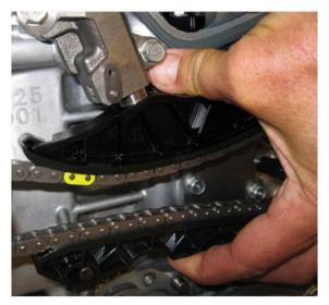
• Rotate the crankshaft COUNTER-CLOCKWISE until the crankshaft sprocket timing mark is at the 6:00 position. Position the cam sprocket timing marks as shown below; intake 6:00, exhaust 12:00.
