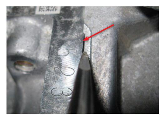
• Once the engine is removed, if you are using a generic engine stand (preferable since engine rotation is necessary), use the four mounting holes on the engine block shown below to mount it. Do not use the studs in the upper oil pan as the upper oil pan has to be removed to access the connecting rod bolts. **NOTE:** The connecting rod bolts are one-time-use and must be replaced.
