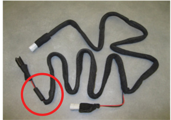
With mini-fuse installed
