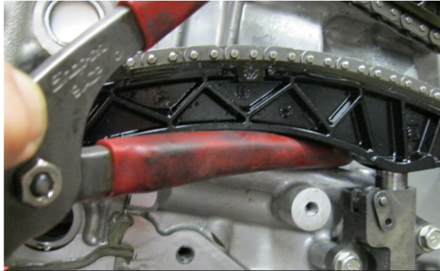
Rubber-coated plier handle inserted between a ledge area on the front of the block and the B1 lower chain guide VERY CAREFULLY lifting upward on the lower guide.
