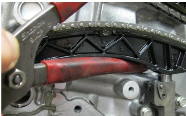
Rubber-coated plier handle inserted between a ledge area on the front of the block and the B1 lower chain guide VERY CAREFULLY lifting upward on the lower guide.
