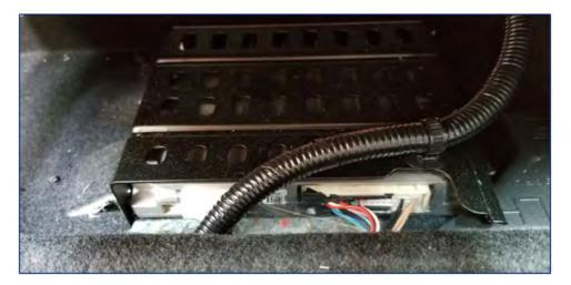
Two lines are used for the interrupt, where one is for NAV and the other one is for the phone. Two are used for CAN, while the other two are used for entertainment (radio, media, etc.).
