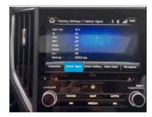
Rotate the steering wheel to confirm the number is changing with the steering wheel rotating.
