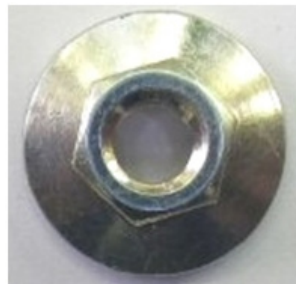
Revised Nut, 15mm diameter flange surface
