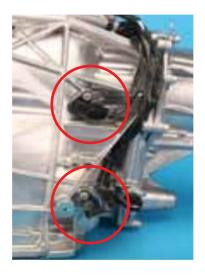
**NOTE:** The sealing o-ring is a one-time use part. Therefore, any time the revolution sensor is removed, the sealing o-ring must be replaced.
