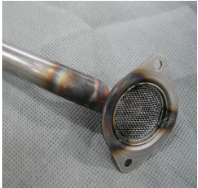
Oil Pick Up Tube/Filter Screen Assembly
