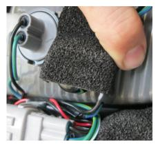
• Tuck the LED harness past the sealing material into its corresponding retaining groove.
