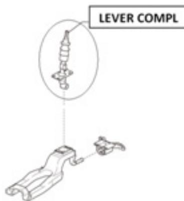
Once the customer's concern has been confirmed to be associated with the shift lever, replace the lever assembly following the service procedure outlined in the applicable Service Manual.
