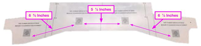
**TIP 2:** The Trailer Hitch Fascia Panel Template (SOA554002) is made from a heavier gauge paper that provides added rigidity. Pre-bending the template in the highlighted areas pictured below can help provide extra flexibility. Bend the template in both directions along the indicated lines.
