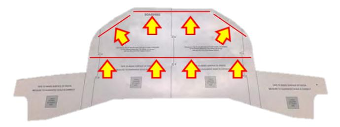
**TIP 3:** Use both hands to press down on the template as shown in the photo below. A helper is recommended for taping down the template or tracing with a marker while being held in place. Use a sharp utility knife to **CAREFULLY** cut the bumper fascia.
