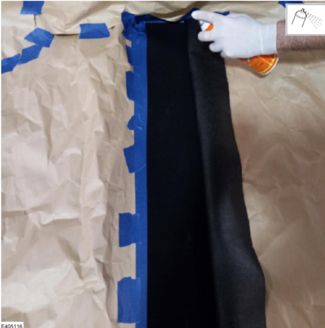
Figure 5 - Showing a properly covered area ready for spray adhesive
