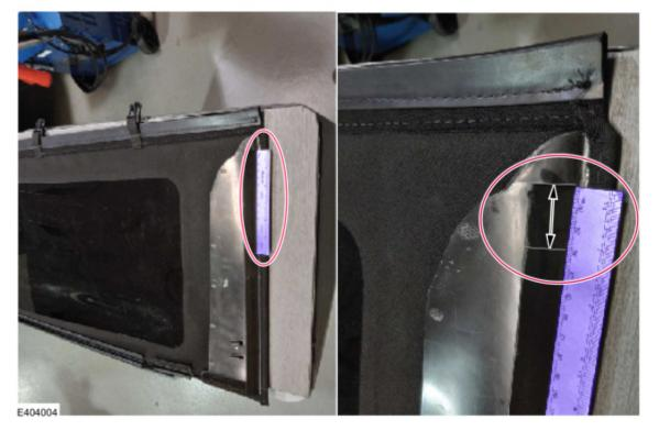
(5). Grab one felt strip (Figure 24, Callout 1) and peel the paper backing off, exposing the adhesive underneath. Install the felt on the previously marked line, keeping it centered on the channel. (Figure 30)
