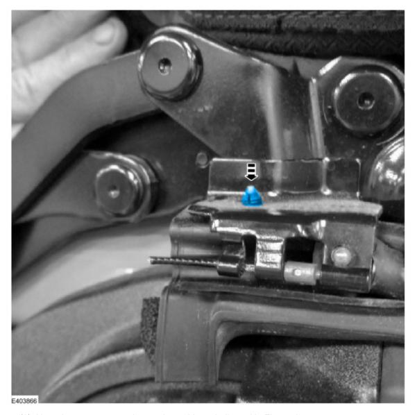
(2). Use wire cutters to cut the tension cable as indicated in Figure 4.
