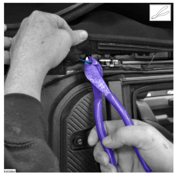
(2). Dislodge the rear spring and completely remove and discard the rear tension cable. (Figure 2)
