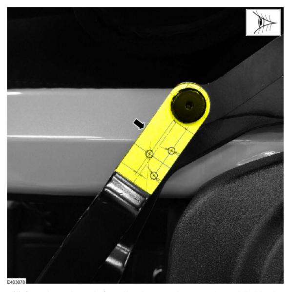
(4). Center the template on the frame. Use a hammer and center punch to mark the 3 locations on the frame to be drilled. (Figure 16)
