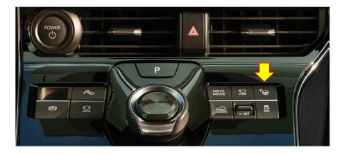
(a) Switch the power switch to the "ON" mode, Press the Parking Assist Button.
