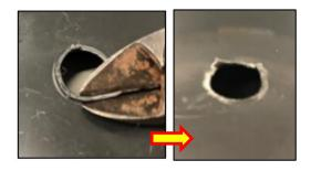
**CAUTION:** Be sure the protrusions are trimmed flush. The remaining protrusion height MUST be less than 2mm to provide proper fitment.
