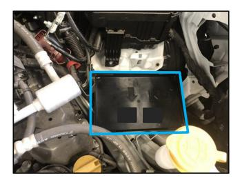
**STEP 4:** Install the original battery cover to the new replacement battery. Confirm the bottom of the cover is aligned flush with the bottom of the battery.
