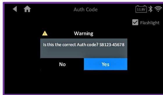
**NOTE:** In a case when the QR Code is entered from the DSS-5000, a Warning screen will display to confirm the Authorization Code for the vehicle being tested. Click “Yes” if the code is correct.
