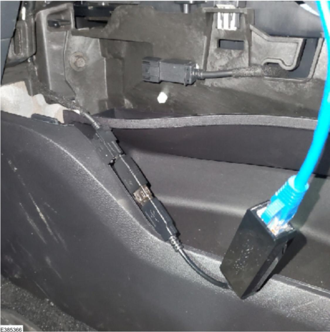
Figure 26 - F-150 with SYNC media hub without center console
