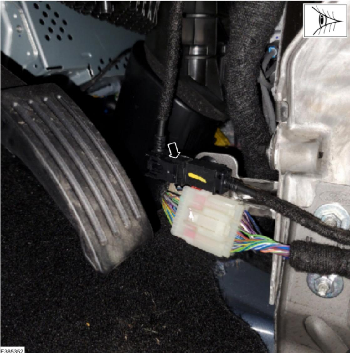
(2). For F-150 vehicles with a SYNC media hub and center console, remove the floor console lower left hand trim panel and disconnect the APIM in-line USB connector. Refer to Step 5 in Workshop Manual (WSM), Section 501-12 floor console removal. (Figures 4-6)
