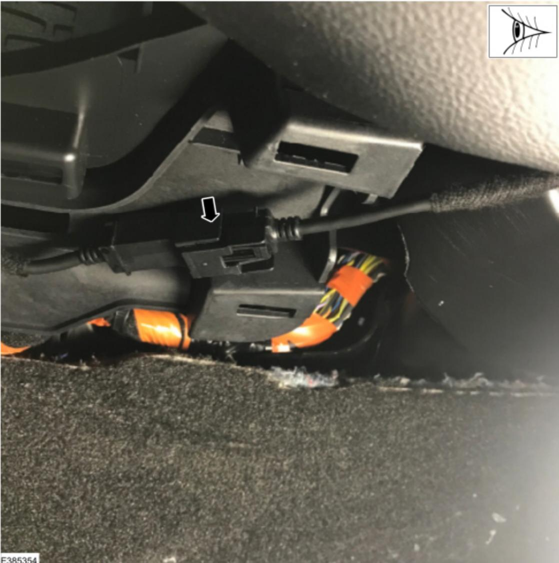
(5). For Edge vehicles, remove the SYNC media hub and disconnect the mini-USB connector on the back of the media hub. Refer to Step 1 in Workshop Manual (WSM), Section 415-00 Media Hub removal. (Figure 11)
