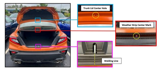
When installing the new seal, confirm the trunk lid center hole, the weather strip center mark and the welding line are all aligned with one another as shown below.
