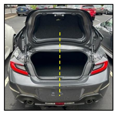
Confirm the entire weather strip is fully seated onto the body flange in all areas.
