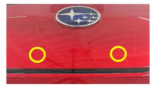
b) Align the dimples with the license plate bracket mounting holes as shown below.
