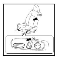
**(f)** Push and hold the **REAR** portion of the "Slide & Vertical Power Seat Switch Knob" to lower the seat position. HOLD the switch for one second after the seat has reached the lowest position.
