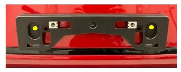
c) Using the supplied self-taping screws, mount the bracket to the bumper while maintaining proper alignment.
