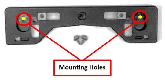
**a)** Locate the dimples located on the front bumper assembly (circled in the image below). These dimples will align with the mounting holes on the front license plate bracket.
