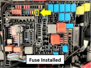
**NOTE:** With the DC CUT FUSE (30A) removed, diagnostic trouble codes (DTC) can be detected when the ignition is turned on during transportation. Clear all DTCs using Global Tech Stream (GTS) after confirming that there are no malfunctions on the vehicle.
