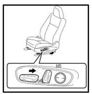
(e) Push and hold the "Reclining Power Seat Switch Knob" to the forward position. HOLD the switch for one second after the backrest has reached its most forward position.
