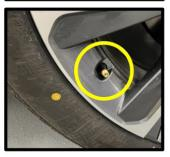
**NOTE:** If some transmitters are not activating, attempt to repeat the process after rotating the affected tire(s) 90 to 270 degrees.
