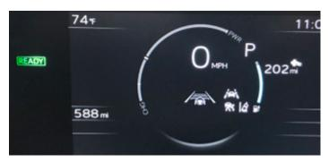
• Every month, check if the battery charge warning light appears on Multi-Information Display. If the warning is illuminated, charge the vehicle using a Level 2 (240-Volt) charger with the charging limit set to 50%.
