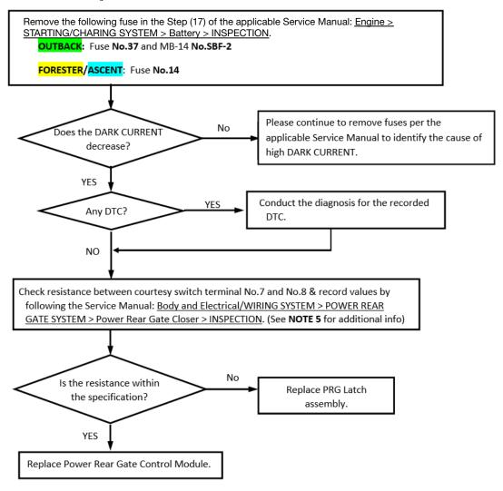
**NOTE 5)** How to check resistance between terminals for Courtesy Switch.
