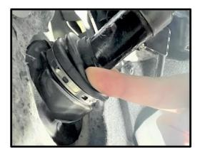
**STEP 3:** Using a lint free cloth, remove any old grease from the steering joint shaft and dust seal.
