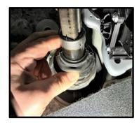
**STEP 2:** Push the dust seal in a downward direction away from the steering wheel. This will allow the old grease to be exposed.
