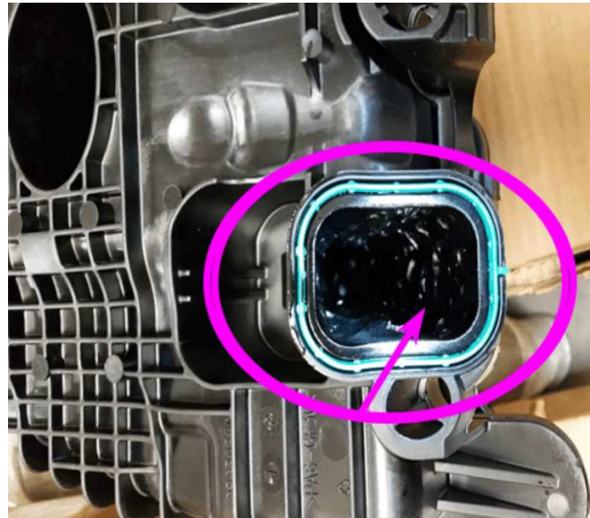
View of Broken Valve that Blew Debris Back into the Intake from the Combustion Chamber
