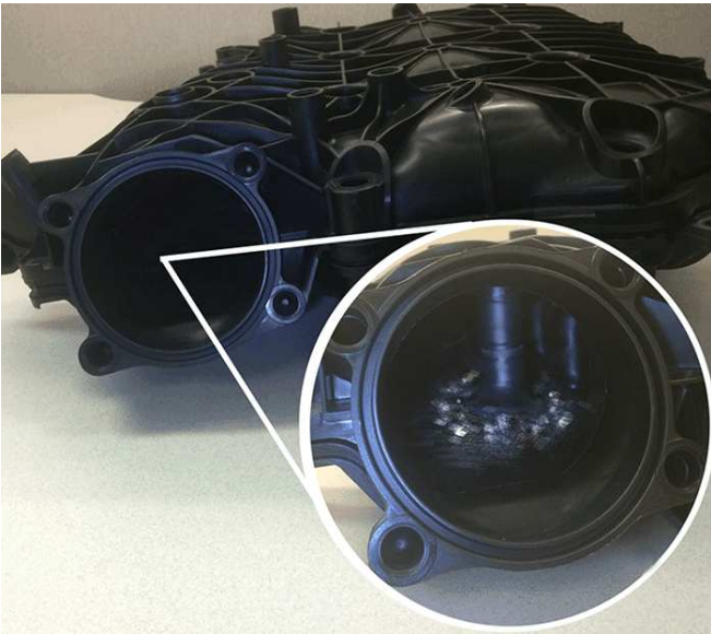
View of Debris in Plastic Intake Manifold – Throttle Body Opening
