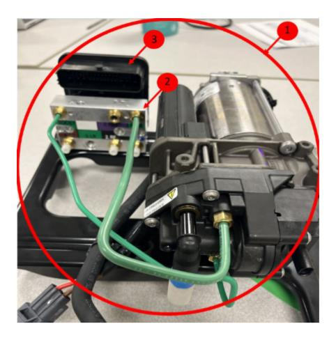
Items 2 and 3, shown above and below, can be replaced separately from the complete Automatic Level Control Module assembly.
