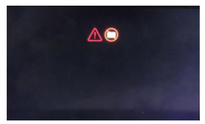
The VPM does not monitor the left, right or front cameras with a rolling counter. These camera's will display in black on their perspective side if there is an issue.
