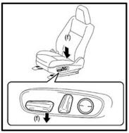
**(g)** Push and hold the **FRONT** portion of the "Slide & Vertical Power Seat Switch Knob" to lower the seat position. HOLD the switch for one second after the seat has reached the lowest position.
