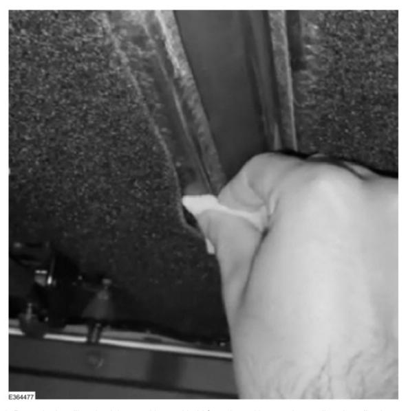
**3.** Press the headliner back into position and hold for at least 40 seconds too allow the adhesive to set. (Figure 3) Figure 3
