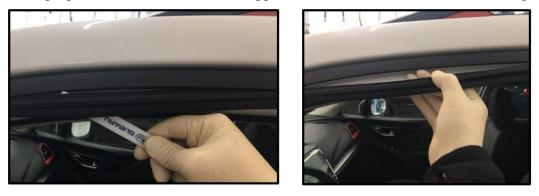
**STEP 5:** Pull the rear section of the seal out by hand while applying forward pressure to the window glass. This will allow less resistance. With the rear section removed, the front section of the seal has less tension, allowing an easier removal. Remove the front section by pulling it out of the channel.
