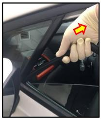
NOTE: SOA glass cleaner (SOA868V9130) or equivalent can be used as an installation lubricant.
