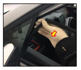
**STEP 7:** Once the seal is pushed down far enough, reach through the access hole created by the removed speaker, and pull the seal down to the desired length.
