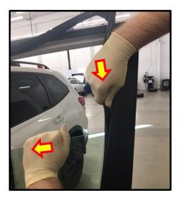
**STEP 9:** The top section of the seal can now be installed. It is Important the alignment of the seal is correct. Use special attention to the front corner glass area of the seal. An alignment hole in the door is matched to bulged portion of the seal.
