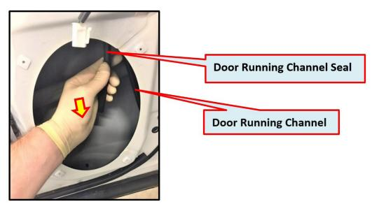
**STEP 8:** While applying forward pressure to the window glass, push the rear section of the seal into the channel until the desire depth is made.
